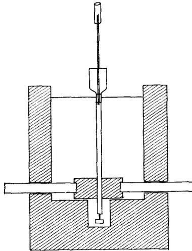
FIGURE 1. The chamber used for the microinjection of radioactive solutions into axons is diagramed schematically. The axon to be injected was tied to a cannula shown at the top end of the axon. A weight was tied to the bottom end and the lower part of the vertically suspended axon was held in the clamp illustrated. A microcapillary was attached to the microliter syringe (not shown) and this was led downward into the axon via the cannula.
