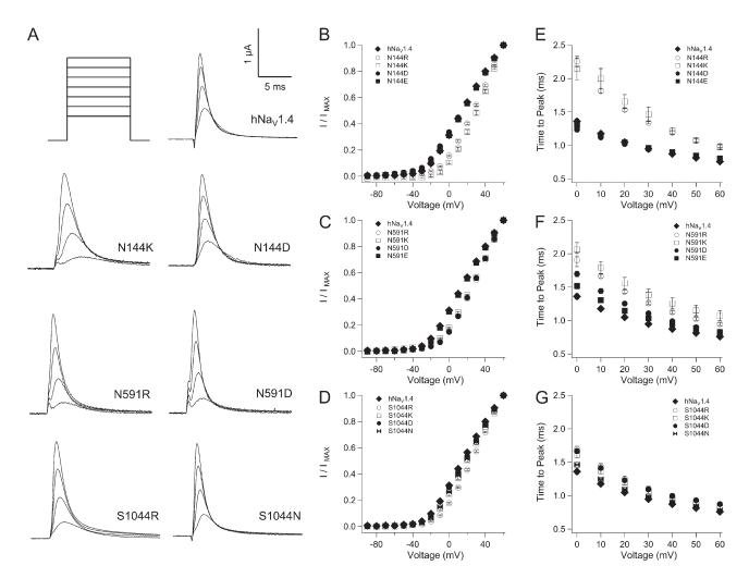
Figure 6. Activation parameters for mutations at S1 HCR locus in  $hNa_V1.4$ . (A) Traces shown are responses to depolarization to 0 mV, 20 mV, 40 mV, and 60 mV for mutations in domains I–III. Plots in B, D, and F show I/V relations for mutations in these domains; plots in C, E, and G show activation kinetics. Values represent mean  $\pm$  SEM (error bars) from 11–24 experiments.
