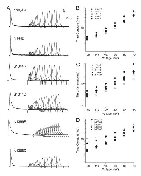
Figure 9. Recovery from fast inactivation for HCR mutations. (A) Traces showing inactivating and recovery sweeps for hNa<sub>V</sub>1.4 and select aspartate or arginine substitutions in domains I, III, and IV. (B–D) Kinetics of recovery at voltages from -120~mV to -70~mV for mutations in these domains. Values represent mean  $\pm$  SEM (error bars) from 10–22 experiments.
