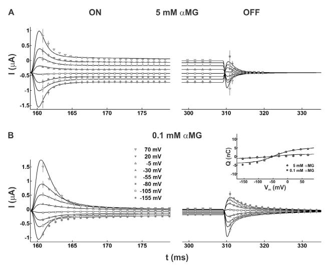
Figure 5. The simulated steady-state and pre–steady-state ON and OFF currents in the presence of 90 mM [Na<sup>+</sup>]<sub>o</sub> and  $\alpha$ MG. Simulated currents obtained with (A) 5 mM or (B) 0.1 mM [ $\alpha$ MG]<sub>o</sub> are compared with experimental data. (Inset)  $Q(V_m)$  curves obtained from integration of the OFF transient currents in the presence of 90 mM [Na<sup>+</sup>]<sub>o</sub> and 5 mM or 0.1 mM [ $\alpha$ MG]<sub>o</sub>.
