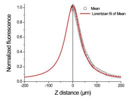
**Figure A1.** Fluorescence intensity depth profile of the objective (USAPO 100XO; Olympus) used in the current experiments. Data points represent normalized mean fluorescence (three trials). The data symbols span the error range.
