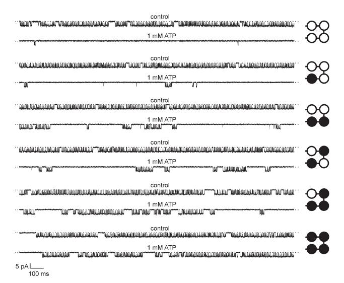
**Figure 4.** Single-channel recordings. Single-channel currents recorded from inside-out patches at −60 mV in the presence or absence of 1 mM ATP. The composition of each tetramer is shown schematically on the right. Open circles, WT subunits; filled circles, Kir6.2-K185E subunits. The dotted line indicates the zero current level.
