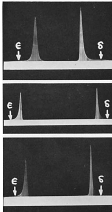
FIG. 5. Moving boundary electrophoretograms of the RJ  $\gamma$ M-globulin preparation at 0.15 ionic strength (0.13 M KCl and 0.02 ionic strength buffers). Top, pH 3.9 sodium formate; middle, pH 8.0 Tris-HCl; and bottom, pH 10.0  $\text{Na}_2\text{CO}_3$ - $\text{NaHCO}_3$ . The times of electrophoresis were 300, 250, and 220 min at potential gradients of  $2.0 \text{ v cm}^{-1}$ .
