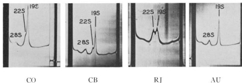
FIG. 1. Sedimentation diagrams of three  $\gamma$ M-globulin preparations CO, CB, and RJ containing various amounts of the 22S component and one (AU) which lacks this material. The direction of sedimentation is to the left and the pictures shown were taken 32 min after reaching speed (59,780 RPM.).
