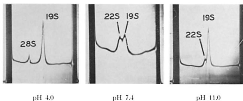
FIG. 3. The effect of pH on the sedimentation properties of RJ  $\gamma$ M-globulin. The experiments were carried out on 1.2% solutions of protein at 20°C. The direction of sedimentation is to the left and all photographs were taken 24 min after reaching speed (59,780 RPM.).
