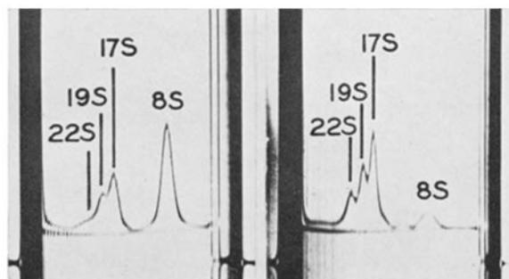
FIG. 6. The sedimentation diagrams of the reaggregated RJ  $\gamma$ M-globulins produced from, left, L-cysteine; and right, 2-mercaptoethanol reduction products. The photographs shown were taken 24 min after reaching speed (59,780 RPM). The experiments were performed at 20°C in 0.15 ionic strength (0.02  $\mu$ , pH 7.4 potassium phosphate buffer and 0.13  $\mu$  KCl).
