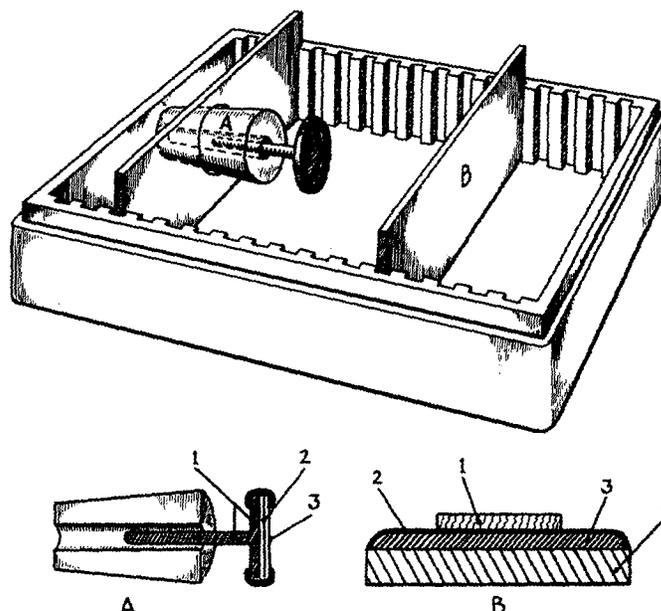
TEXT-FIG. 1. The apparatus for alphasradiography: *A*, rubber stopper mounted on aluminum plate and bearing alpha source: 1, platinum plated metal support; 2, polonium coat; 3, mica cover. *B*, target: 1, tissue section; 2, celloidin coat; 3, nuclear emulsion; 4, glass slide.
