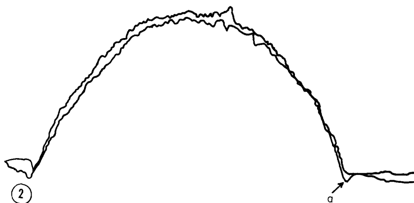
FIGURE 2 Two densitometric traces across perpendicular diameters of drop A seen in Fig. 1. The dip in the densitometer curve (a) is an edge anomaly produced by light refraction. \times 1 .
