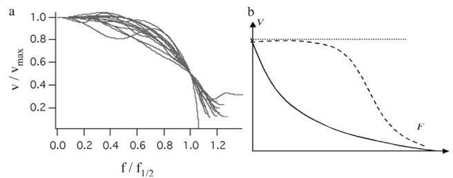
**Figure 5. Experimental data and theoretical prediction of different models.** (a) Normalized force-velocity relation. (b) Force-velocity relations predicted by the ratchet model (solid line), hypothetical stepping motor model (dashed line), and autocatalytic branching model (dotted line).
