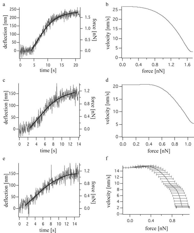
Figure 3. **Three representative deflection/force versus time curves and corresponding force-velocity curves.** (a, c, and e) Deflection/force versus time curves for the lamellipod hitting the cantilever. (b, d, and f) Corresponding force-velocity curves for each example on the left. Representative error bars were calculated as described in Materials and methods for every 10th data point.
