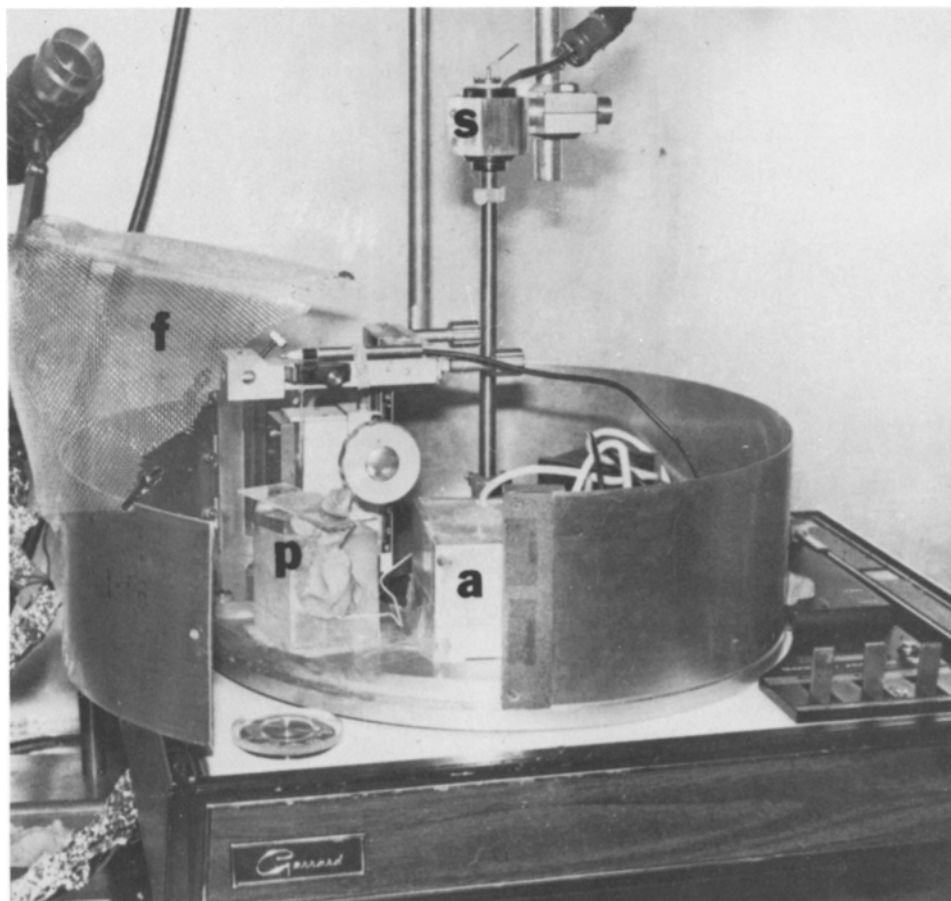
FIGURE 2. Photograph of modified Garrard turntable and recording apparatus. (f) Faraday cage. (p) pedestal for preparation. (a) amplifier. (s) slip rings.
